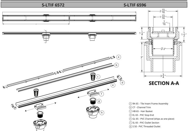
h 2 inch clamp down drain assembly Not included in kit SKU. (Material can be Cast Iron, ABS, or PVC)
