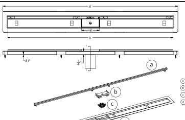
GRATE CAN BE ADJUSTED UPWARDS AN ADDITIONAL 1/2"
